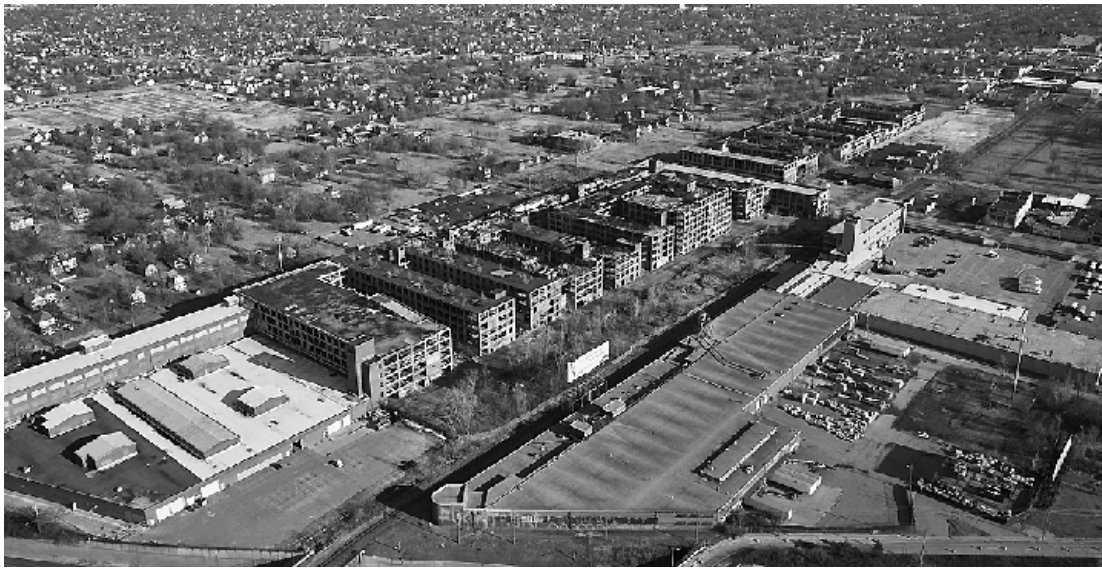
A MODERN VIEW of the Packard Plant ruins in Detroit. Designed by Albert Kahn with a groundbreaking reinforced concrete structure, the plant made Packard cars until 1956, except during World War II, when it made P-51 Mustang fighter engines. In its heyday, the plant employed 40,000 workers. For a time until the late 1990s, the site was used for storage, chemical production, and even parties, before closing for good in 2010, as scavengers, graffiti artists and paintball players had the run of the grounds. The plant employed as many as 40,000 workers.
