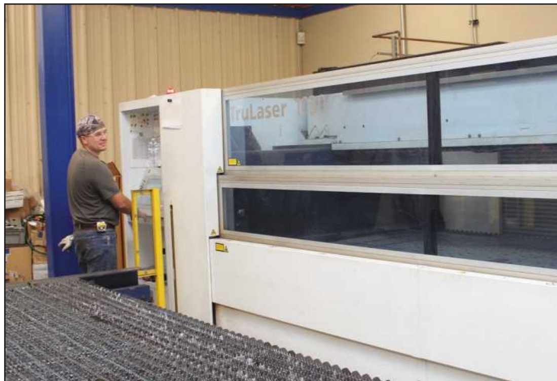
SETTING UP A True Laser 1030 cutting machine for work on a platform is Dan McLeod of Sheet Metal Workers Local 7. He's working at the Shouldice shop in Battle Creek.
