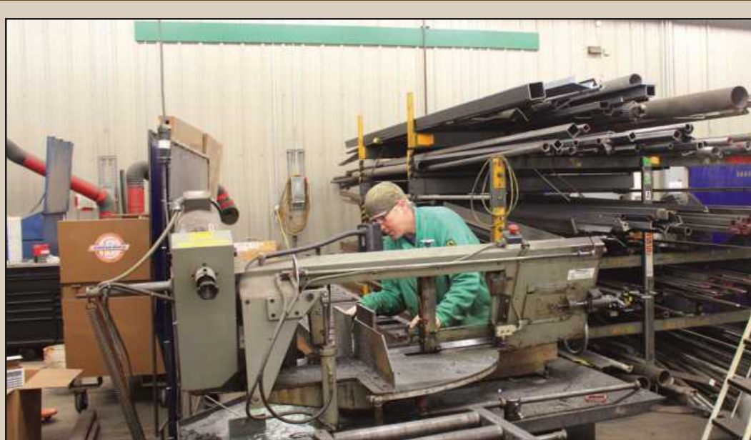
FABRICATING A HAND RAIL section at the Shouldice shop in Battle Creek is Jason Emmons of Sheet Metal Workers Local 7.
