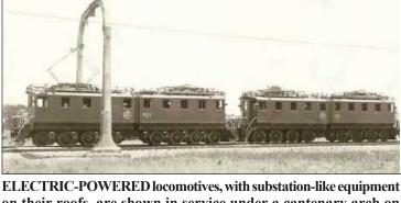
on their roofs, are shown in service under a cantenary arch on Ford's Detroit, Toledo and Ironton line on July 29, 1928.
